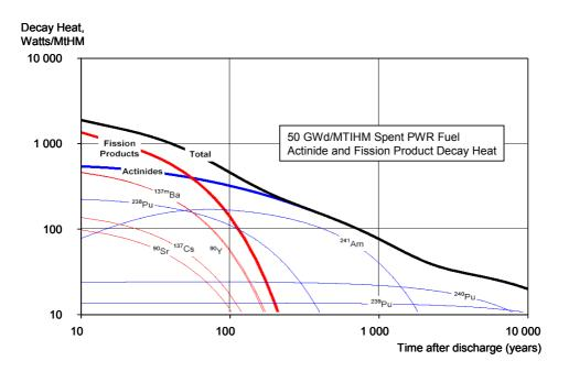
Figure 29: Contribution of each component of used fuel to the decay heat
