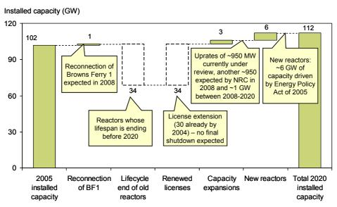
Figure 23: Expected nuclear installed capacity in 2020
