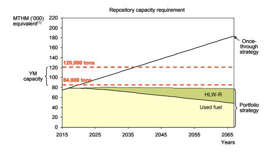
(1) Equivalent to MTHM ('000) of used fuel disposed in the repository (i.e., HLW-R takes only ½ of the space from equivalent used fuel)
