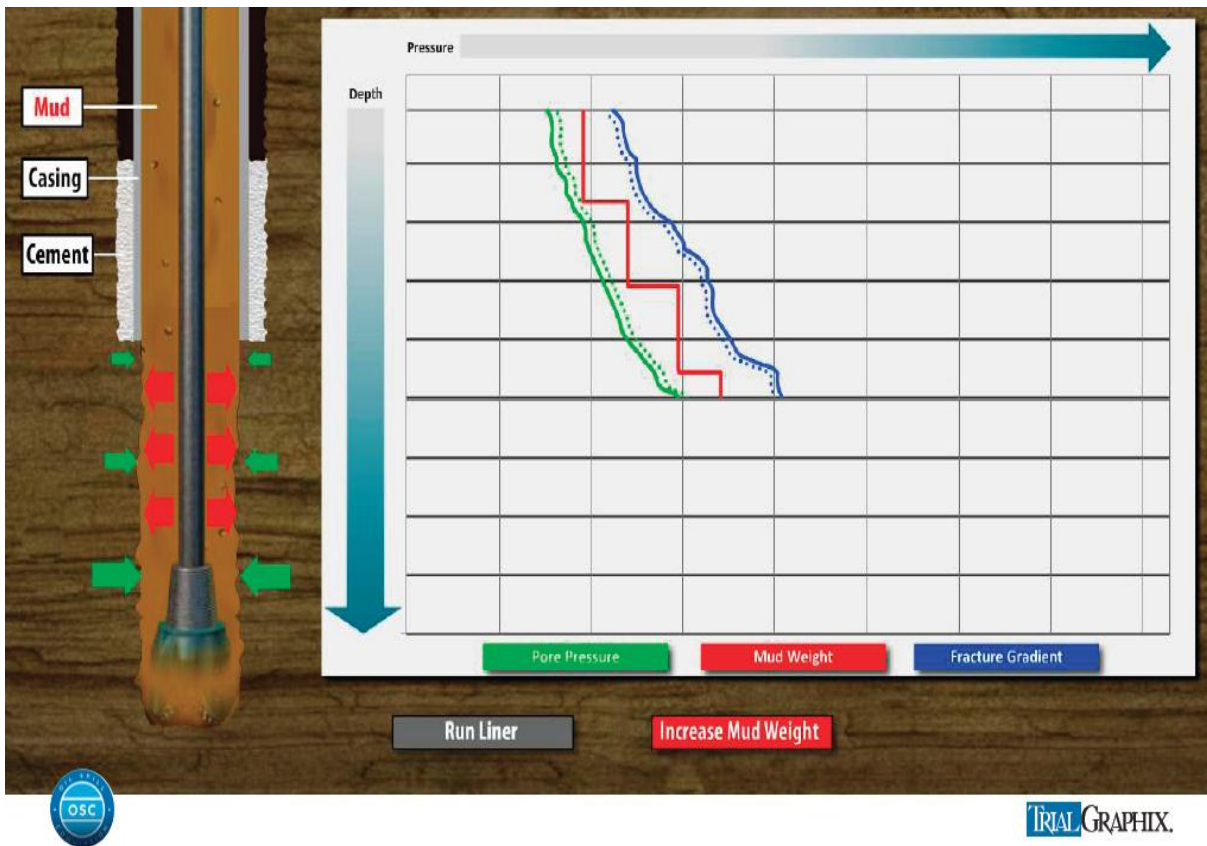
Figure 1.6 – Illustration of Borehole Pressures and the Drilling “Window”. 24
