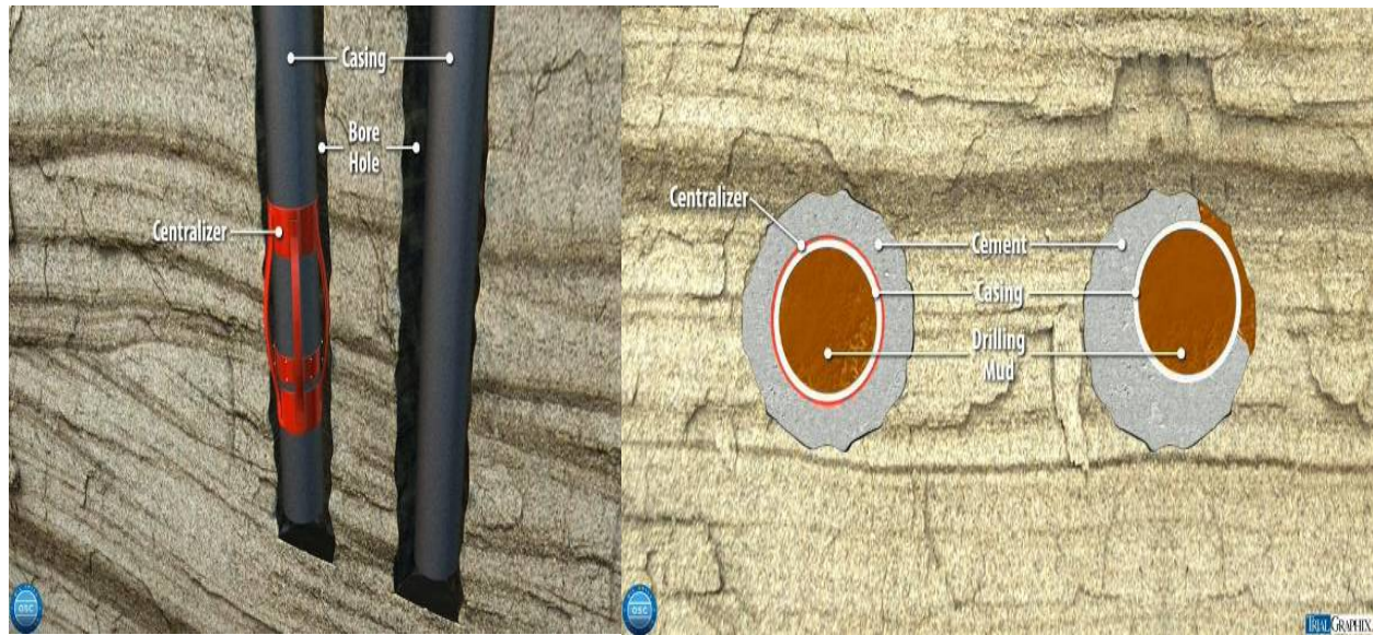
Figure 1.16 – Centralizers. 50
