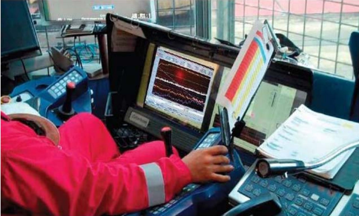
Figure 1.21 – View of the driller's data-panel. 99
