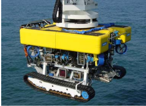
Exhibit 7.2. Remotely operated vehicle for subsea cable operations. 30
