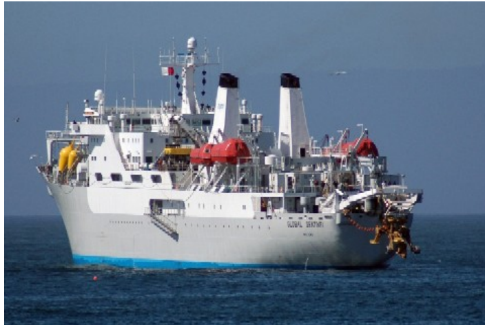
Exhibit 7.1. Cable-installation vessel. Note remotely operated vehicle suspended from the aft gantry. 26
