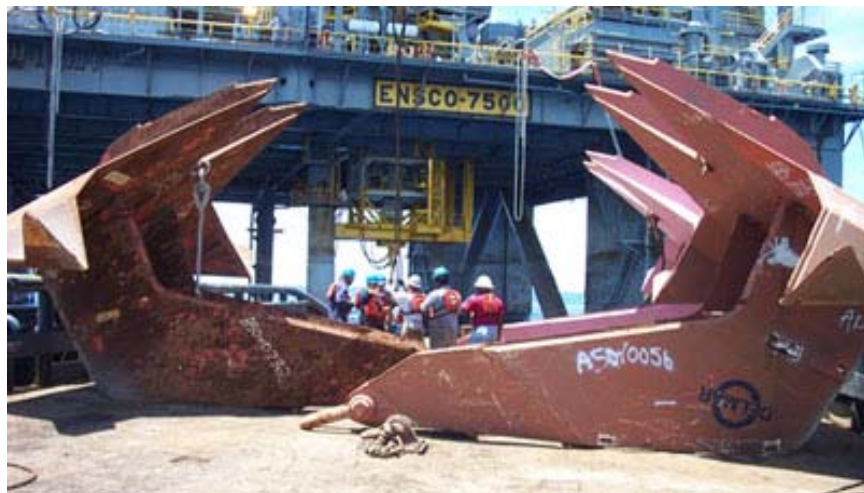
Exhibit 9-11. Large single-fluke anchors used to “permanently” anchor offshore structures (Delmar 2009a).
