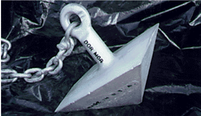
Exhibit 9-14. The Dor-Mor pyramid mooring anchor can require breakout tension greater than ten times the anchor weight (Dor-Mor 2009).
