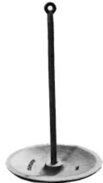
Exhibit 9-13. The mushroom anchor relies on the head becoming buried in sediment. 43
