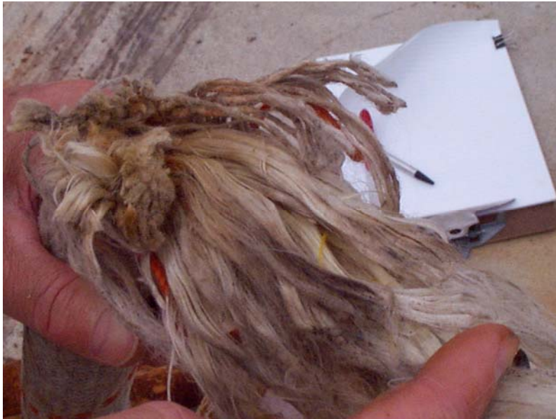
Exhibit 9-21. A polysteel rope half cut (left part of rope) by the sharp edge of the anchor fluke in exhibit 9-12. 53
