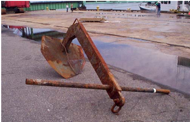
Exhibit 9-12. Medium-size single-fluke drag anchor designed for multi-anchor operations of a subsurface grid into which various structures might be inserted. 42
