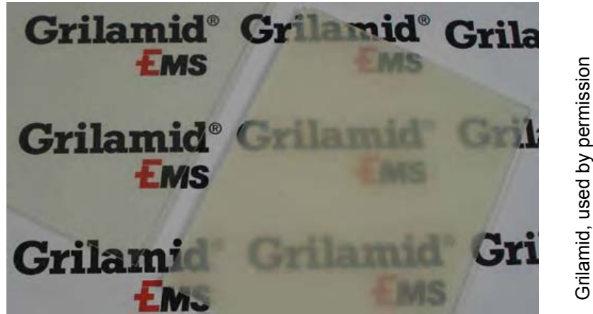
Figure 46. Thermotropic polyamide in clear and scattering states
