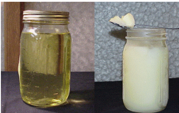
Figure 3.—One issue to address is that regular bio-diesel fuel (left) freezes at the cold (i.e., -20 °C) operating conditions of aircraft (right) (ref. 3).
