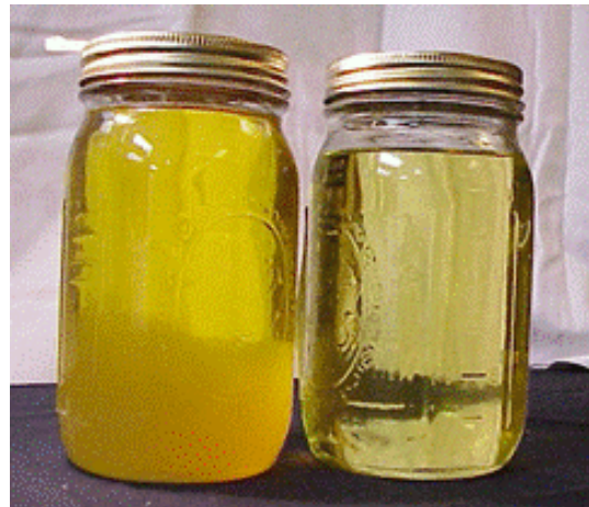
Figure 5.—Biofuel (right) would need to be mixed at a maximum 20 percent ratio to avoid stability issues over time (left) (ref. 3).
