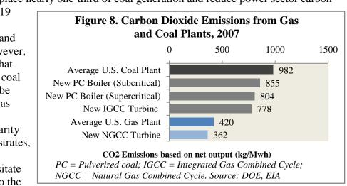
Besides being more efficient and cleaner than their coal counterparts, combined-cycle power plants are also cheaper and quicker to build. A survey of actual fossil, nuclear, and renewable power projects in 2008 determined that natural gas combined-cycle plants had the lowest construction costs of any available generating technology, under half the cost of a new pulverized coal plant and just one-fifth the estimated cost of a new nuclear plant.<sup>37</sup>
