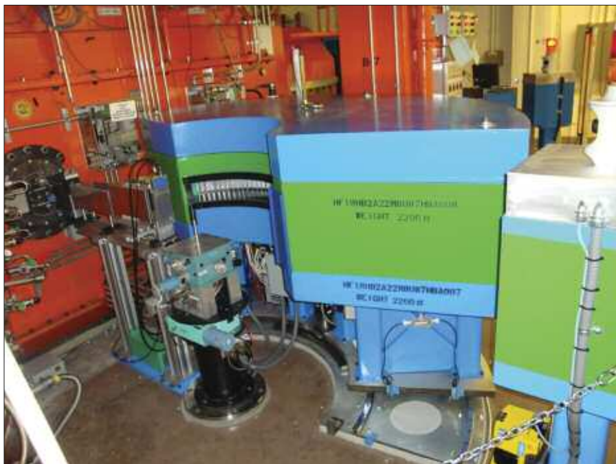
Fig. 6. The new HB-2A Powder Diffractometer at HFIR
