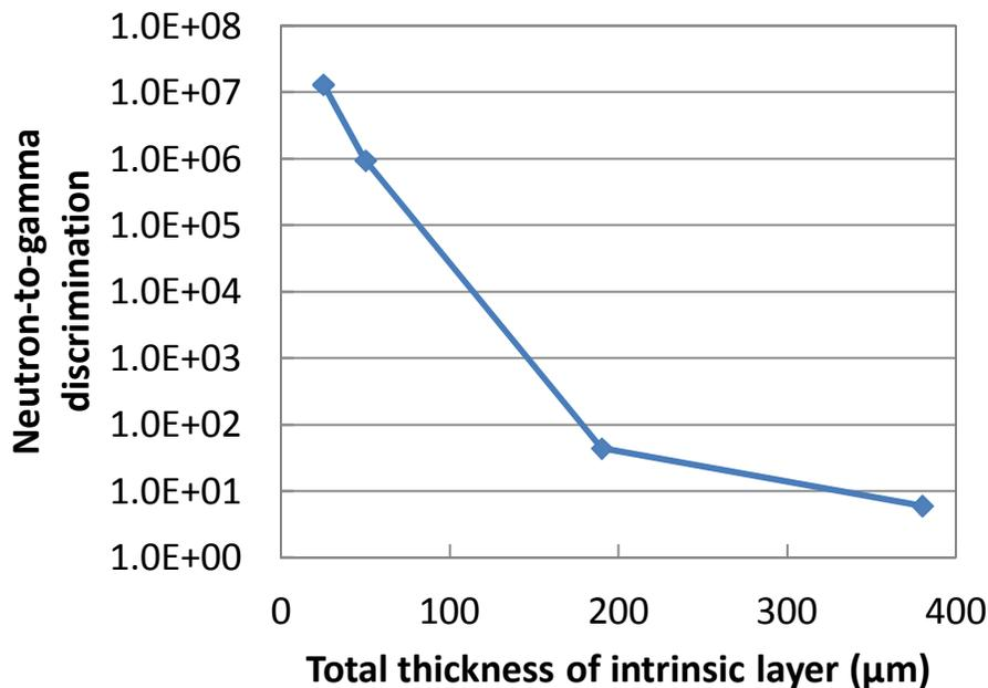
Figure 3 Measured gamma discrimination with gamma energy of 662 keV as a function of total thickness of intrinsic layer (Pillar heights are 25  $\mu\text{m}$ , 50  $\mu\text{m}$ , 50  $\mu\text{m}$  and 50  $\mu\text{m}$  for four samples with 25  $\mu\text{m}$ , 50  $\mu\text{m}$ , 190  $\mu\text{m}$  and 380  $\mu\text{m}$  intrinsic layers respectively)
