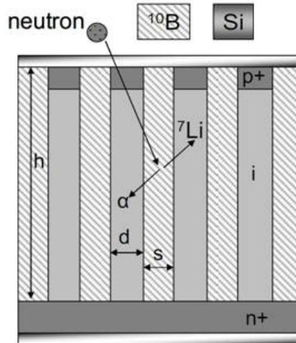
Figure 1 Schematic of a pillar structured thermal neutron detector, h: pillar height ( $50 \mu\text{m}$ ), d: pillar size ( $2 \mu\text{m}$ ), s: pillar separation ( $2 \mu\text{m}$ )
