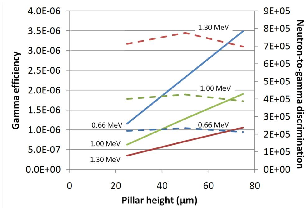
Figure 4 Simulated gamma efficiency (solid lines) and neutron-to-gamma discriminations (dotted lines) for a pillar diameter of 2  $\mu\text{m}$  and pillar separation of 2  $\mu\text{m}$  versus pillar height (LLD setting: 50 keV)
