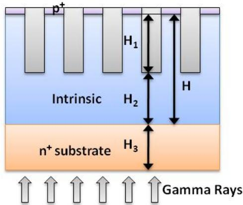
Figure 2 Schematic of a pillar structured thermal neutron detector with gamma radiation
