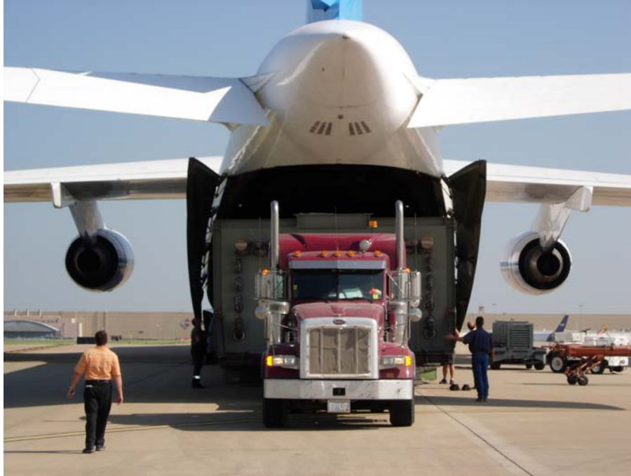
Fig. 2. Russian Antonov An-124 Aircraft (payload 120 tonnes) loading refinery heating unit through the rear door (photo provided by Tailwind Air Charters, Addison, Texas).
