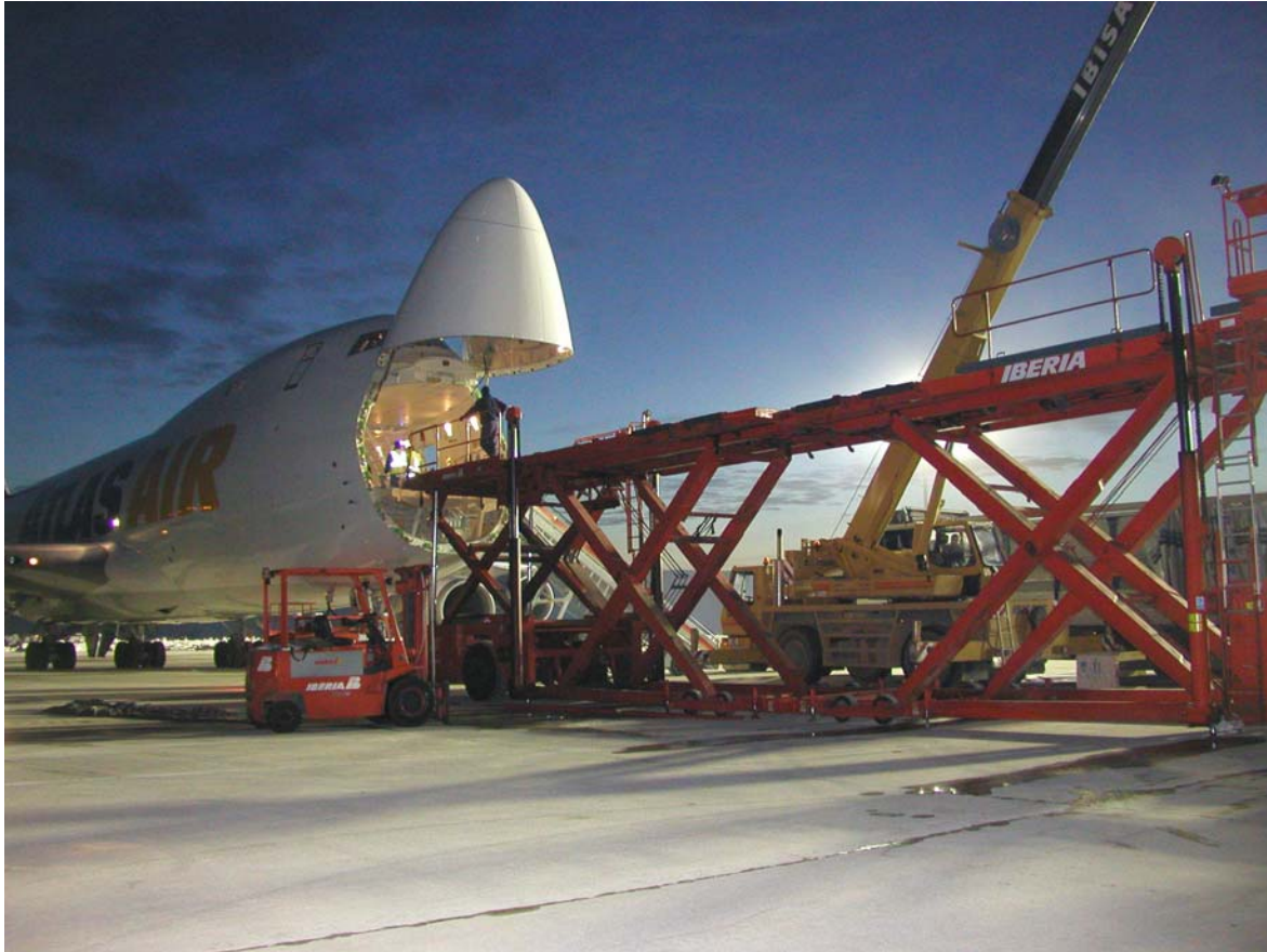
Fig. 1. B747-400F aircraft (payload 112 tonnes) preparing to load a 40-ft-long pipe in Spain (photo provided by Tailwind Air Charters, Addison, Texas).
