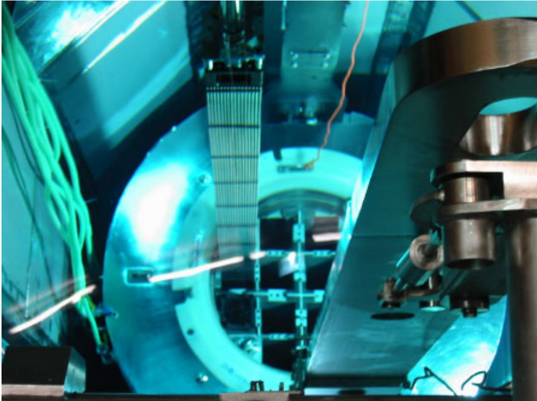
Figure 6a. Loading of spent fuel assemblies in a cask under water (TN13/2).
