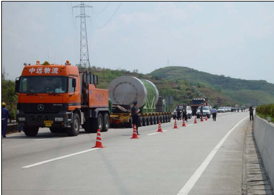
Figure 6. Cask transportation operation (NAC-STC cask from Daya Bay to Lanzhou) 2.
