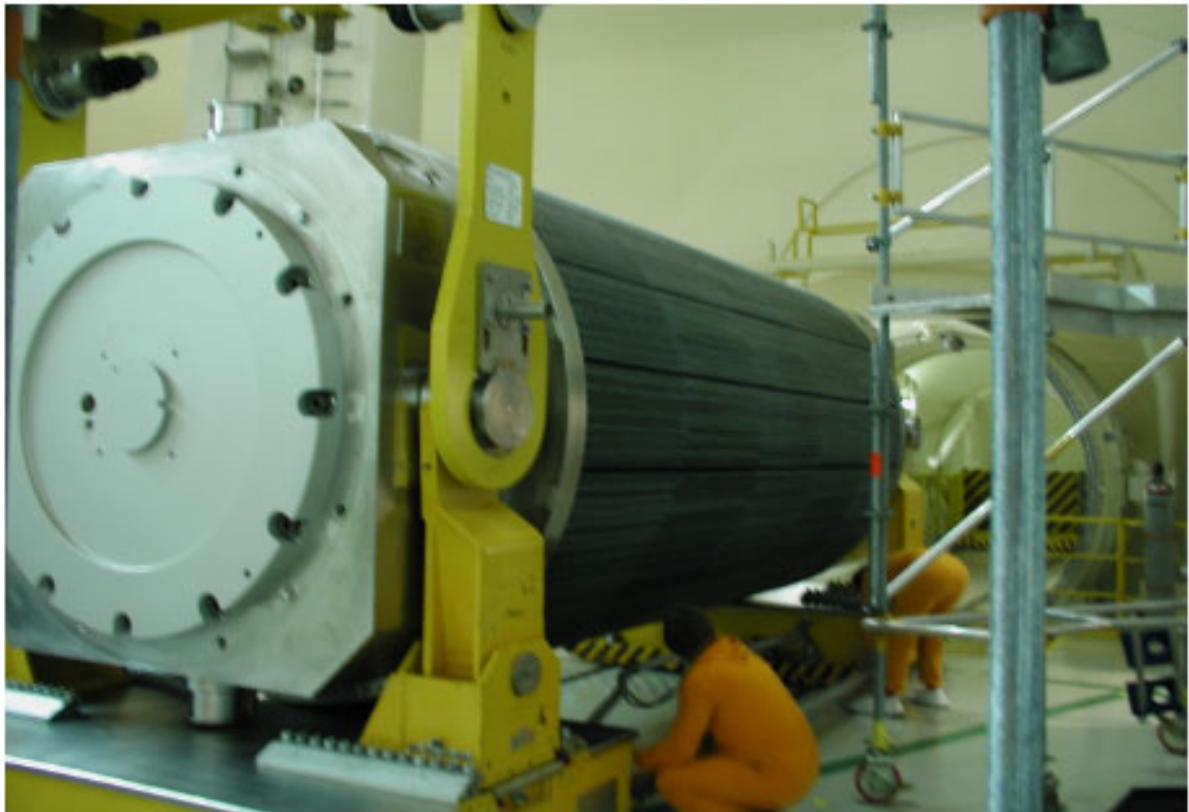
Figure 4. A cask arrival operation for spent fuel transportation (TN-13/2).
