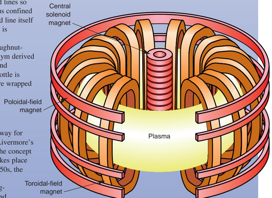
In a tokamak, magnetic fields from surrounding magnets confine a plasma fuel of hot, ionized gas within a hollow, doughnut-shaped vacuum chamber.
