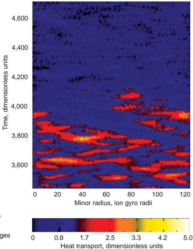
localized changes in the rate of plasma rotation. The flow shear sharply reduces the rate at which heat is transported out to the cold plasma edge by stretching and tearing apart the microturbulence eddies.
