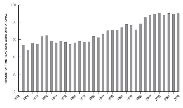
Figure 5. Average Annual Capacity Factor of U.S. Nuclear Power Reactors
