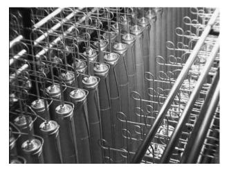
Gas centrifuges used to enrich uranium
