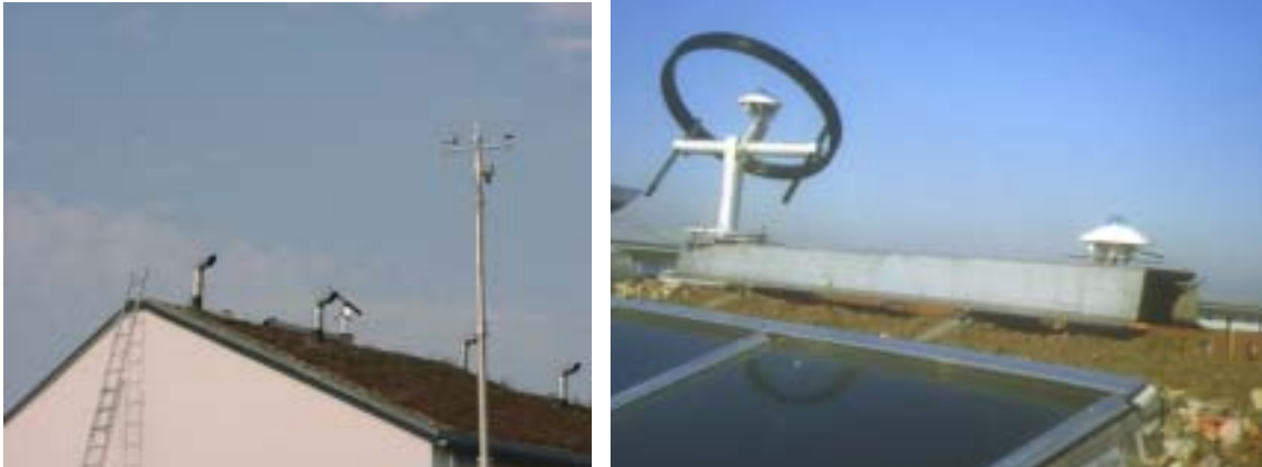
Figure 43 and Figure 44: Weather station in the Passive House estate. Left : Telescope pole with the sensors. Right : Radiation measurement units with and without shadow ring on the ridge.
