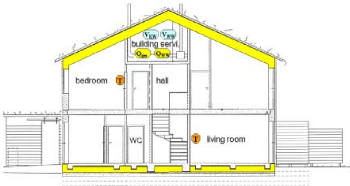
Figure 39: Cut-away section through a terraced Passive House with drawn-in location of the measurement points for the standard measurement (according to [Pfluger 2000]).
