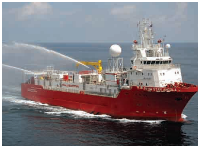
Fig. 2 —Equipped with 8,250 hhp and 15,000 psi-capable pumps and manifolds, Halliburton's Stim Star Angola delivers a wide range of stimulation services offshore West Africa. Photo courtesy: Halliburton.
