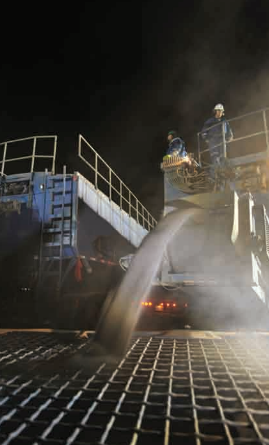
Fig. 6 —Proppant being moved into the hopper for feeding into blender trucks from which the mixture will be pumped downhole during hydraulic fracturing. Location: Haynesville well in northern Louisiana. Photo courtesy: Carbo Ceramics.
