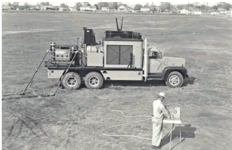
Fig. 6—Vintage 1950s remotely controlled frac pumper powered by surplus WWII Allison aircraft engines.
