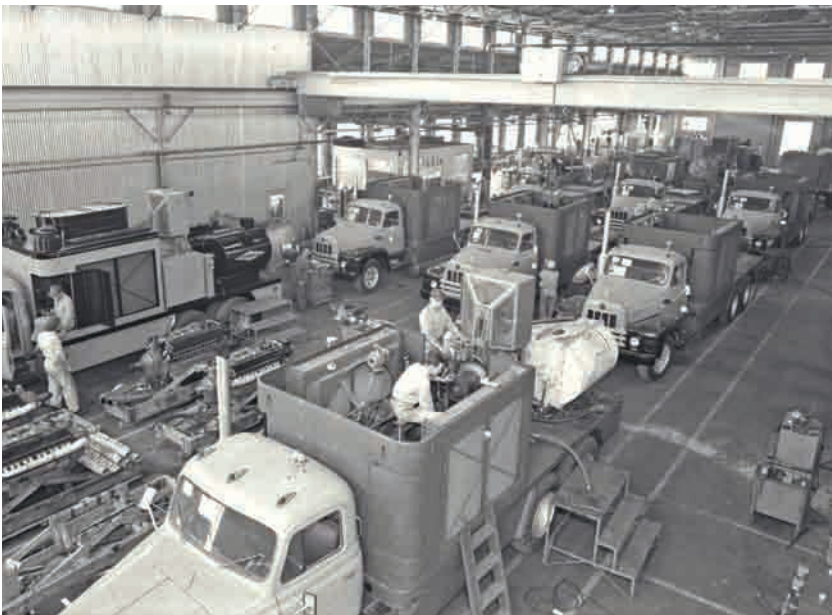
Fig. 3 —A 1955 frac pump manufacturing facility. These remotely controlled pumps were powered by 1,475 hp surplus Allison aircraft engines used during World War II.
