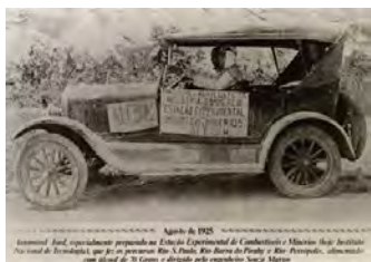
Ford Model T adapted by INT for demonstrations of ethanol use in 1925
