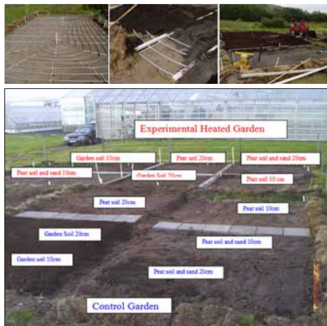
Figure 2: Hveragerdi spiral piping layout (top left), sand over layer construction detail (top center), soil top layer and gravel compaction construction detail (top right), soil depths, types and location (Bottom)
