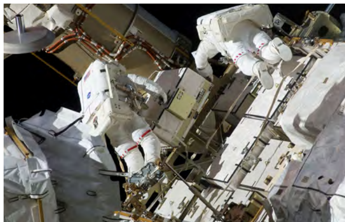
Astronauts work to replace a battery unit during space shuttle Endeavour's STS-127 mission to the space station in July 2009.
