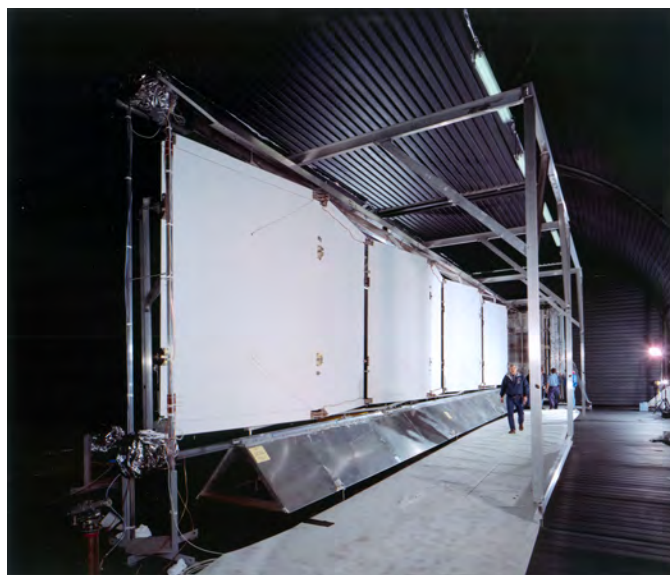
Radiator testing in the Space Power Facility at NASA's Plum Brook Station in Sandusky, Ohio.
