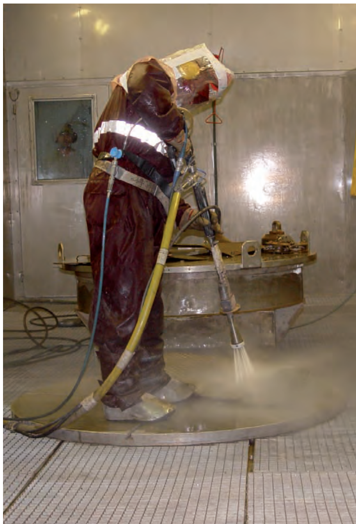
Abb. 24: Full protective clothing during decontamination by high-pressure cleaning
