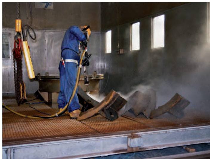
Fig. 26: Decontamination by high-pressure water jet cleaning
