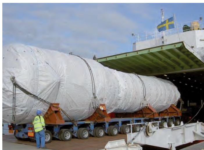
Fig. 30: Transport of a steam generator to Sweden for melt-down
