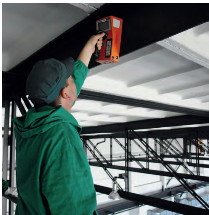
Fig. 16: Measurement to determine a possible contamination
