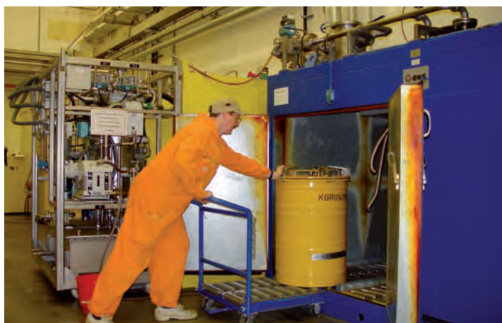
Fig. 39: Conditioning of waste (in-drum drying facility)
