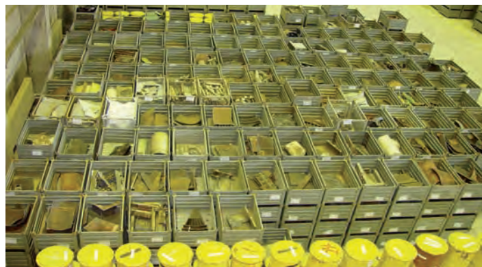
Fig. 32: Boxes with sorted residues for clearance
