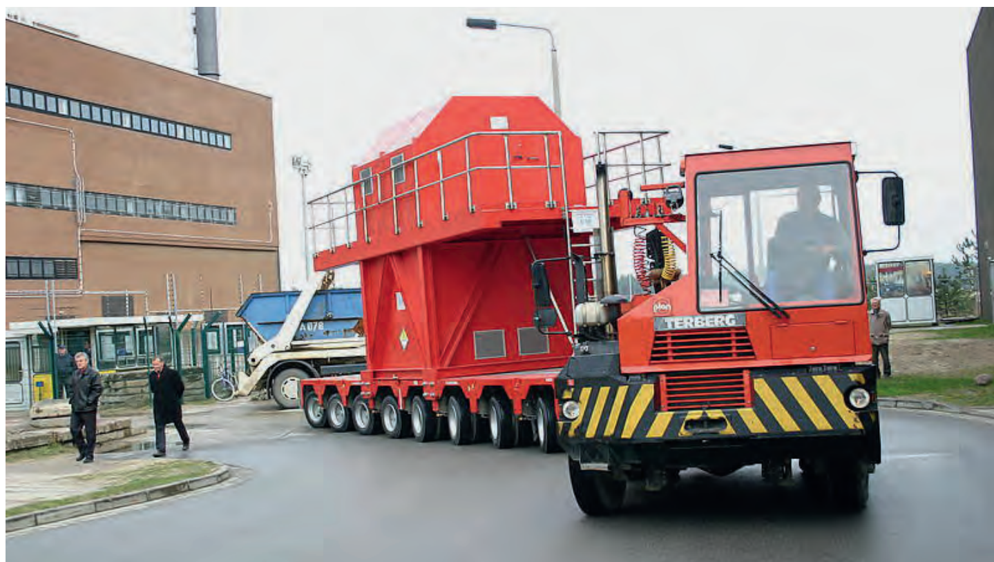
Fig. 21: Plant-internal transport of irradiated fuel assemblies
