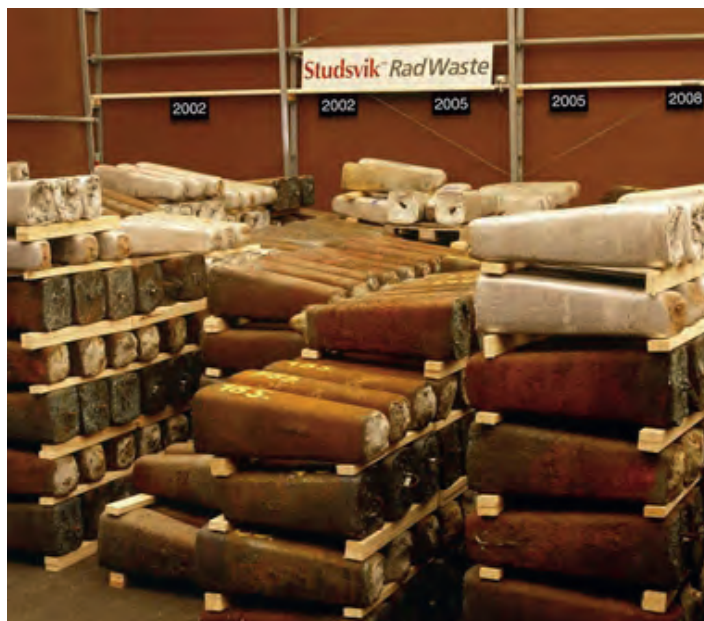
Fig. 37: Decay storage of castings
