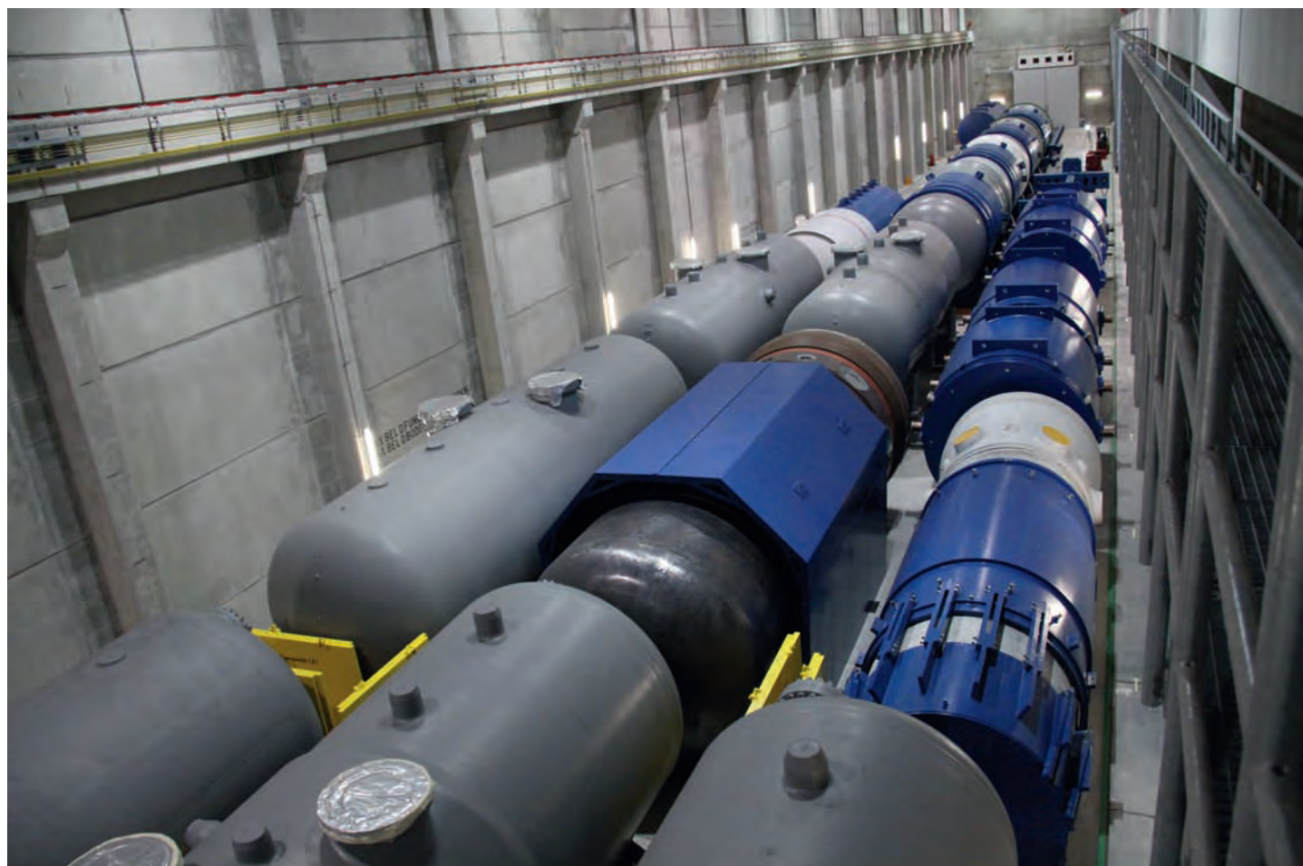
Fig. 42: Decay storage of large components at the Interim Storage Facility North (ZLN)
