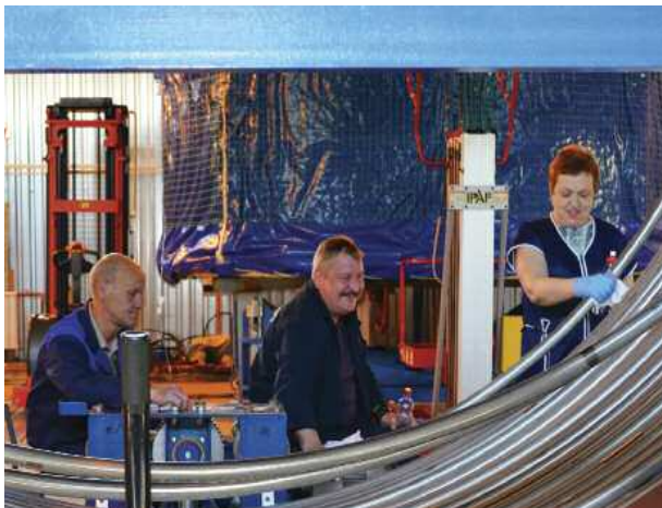
In Russia, the last production length of toroidal field conductor is jacketed and compacted in June. The year 2015 marked the near close of an eight-year procurement campaign, with more than 90% of toroidal field conductor unit lengths produced in the factories of China, Europe, Japan, Korea, Russia and the United States. Photo: ITER Russia
