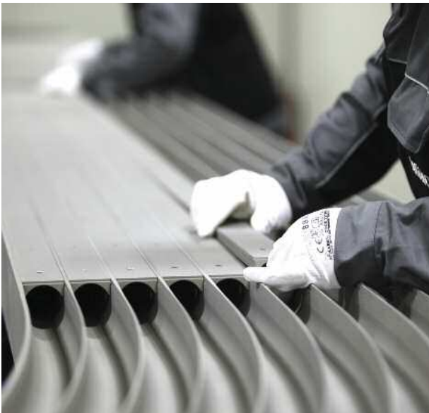
Radial plates have the role of supporting toroidal field conductors within their coils cases. At a manufacturing factory in Europe, technicians fit the cover plate onto one 5m x 16m plate. Photo: F4E
