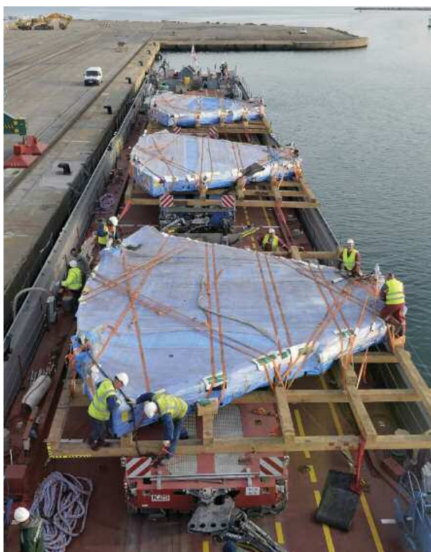
Twelve segments of the massive cryostat are shipped from India to ITER in 2015 -- the very first Tokamak components to reach and be stored on site.
