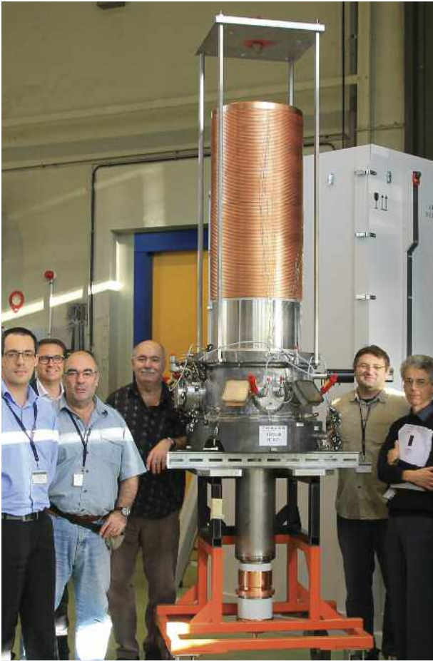
Radio-frequency devices called gyrotrons will generate microwave beams over a thousand times more powerful than a traditional microwave oven. In April, the continuous wave gyrotron prototype successfully passes final factory acceptance tests in Europe. Photo: F4E
