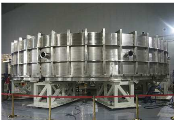
For poloidal field coil #6, which will be manufactured in China under an agreement concluded with Europe, tooling and component qualification is underway. (In the picture: a vacuum chamber for leak tests.)
