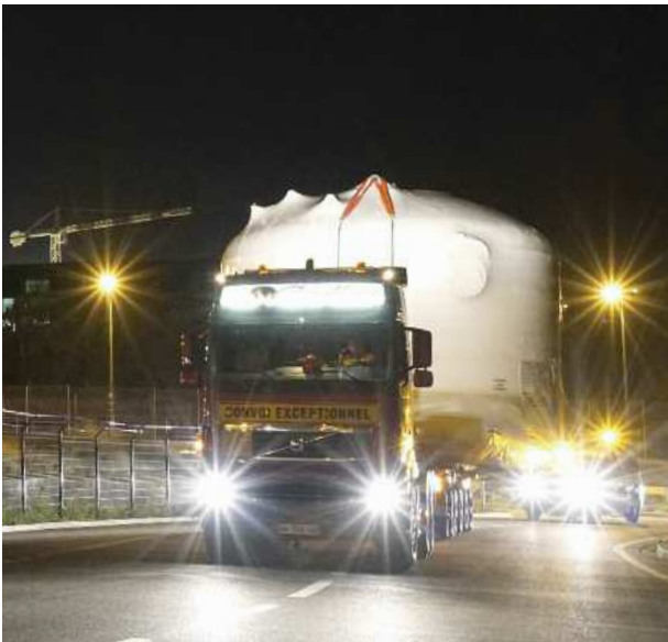
ITER Highly Exceptional Loads travel at night in order to minimize traffic disturbance. Pictured: one of the five stainless steel drain tanks shipped from the US in 2015 for ITER's cooling water system.
