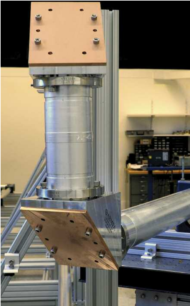
As a contribution to ITER diagnostics, the US is designing seven instruments plus four port plugs. This test stand for the low-field-side reflectometer diagnostic mimics an ITER-like waveguide route. Photo: US ITER
