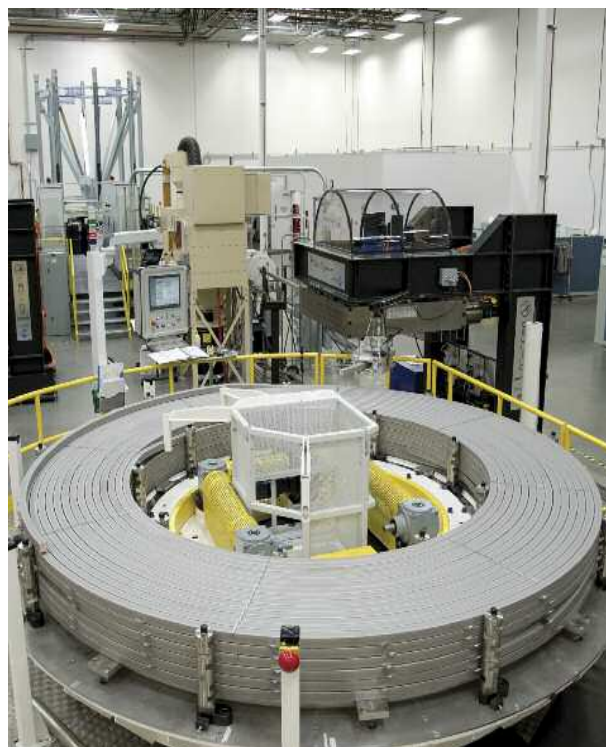
Following the success of mockup winding (pictured) at the central solenoid fabrication facility in the US, winding has begun on the first production module. Photo: US ITER
