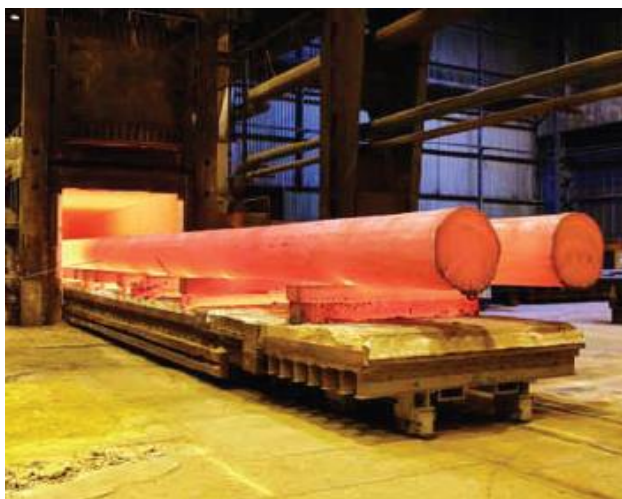
Fig. 9 Heat treatment of longitudinal forgings Maximal dimensions of forgings: of the shaft: D = 3,000 mm, length L = 25,000 mm; rings = 5,000 mm; hollow bodies D = 4,300 mm; circular plates D = 5,500 mm
