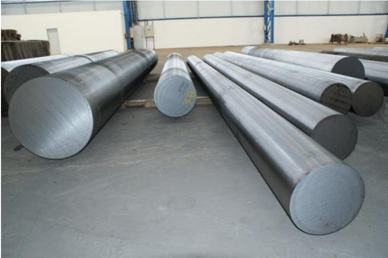
Fig. 13 Round rod forged on the radial forging machine
