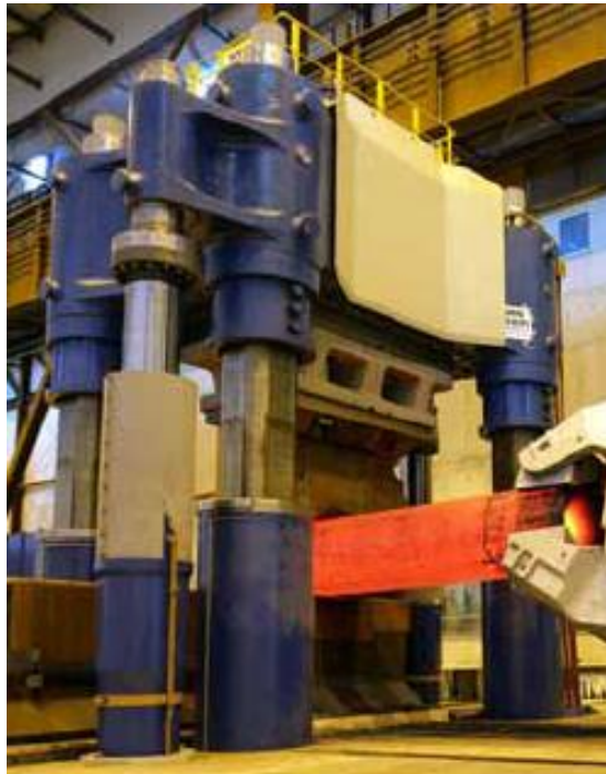
Fig. 8 Hydraulic press of 100 MN for open die forging
