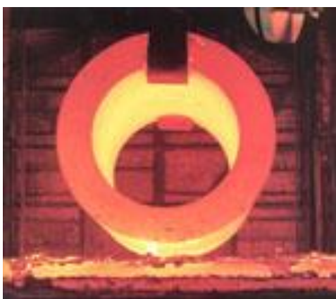
Fig. 10 Heat processing of a roughed-out ring
