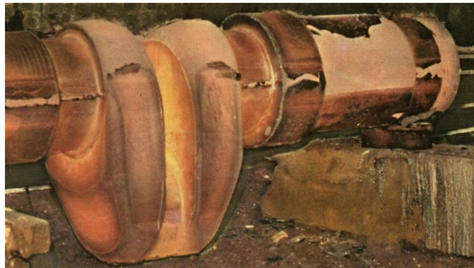
Fig.4 The forging of a ship crankshaft forged by the TR method
