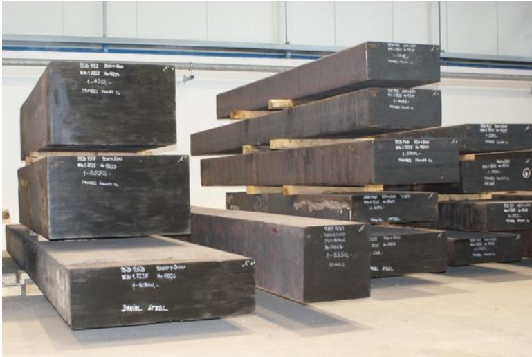
Fig. 14 Large square bars forged in hydraulic presses
