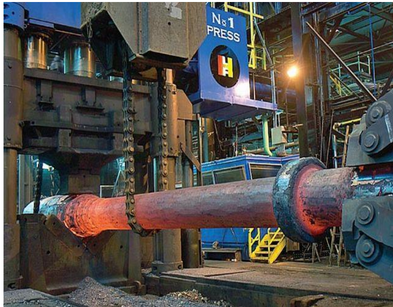
Fig. 12 Ship drive shaft forged on the 100 MN-press in the forge of the Lehigh Heavy Forge
