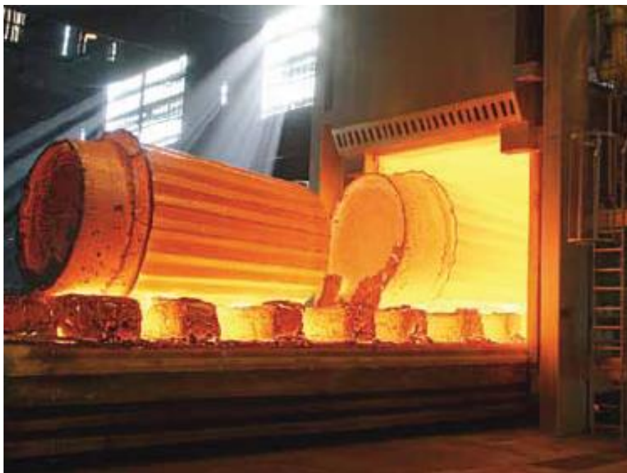
Fig. 11 Ingots heating in a movable-bottom furnace
