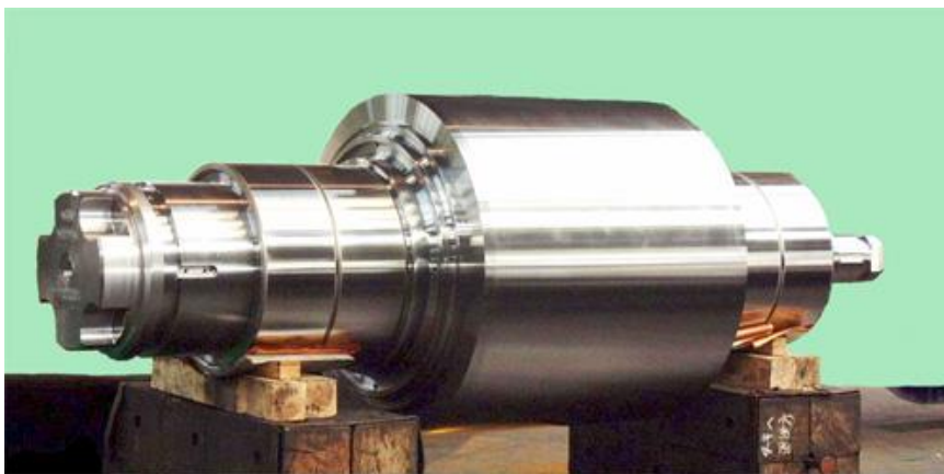
Fig. 3 Machined forging of a roll of steel 5% Cr –Mo
