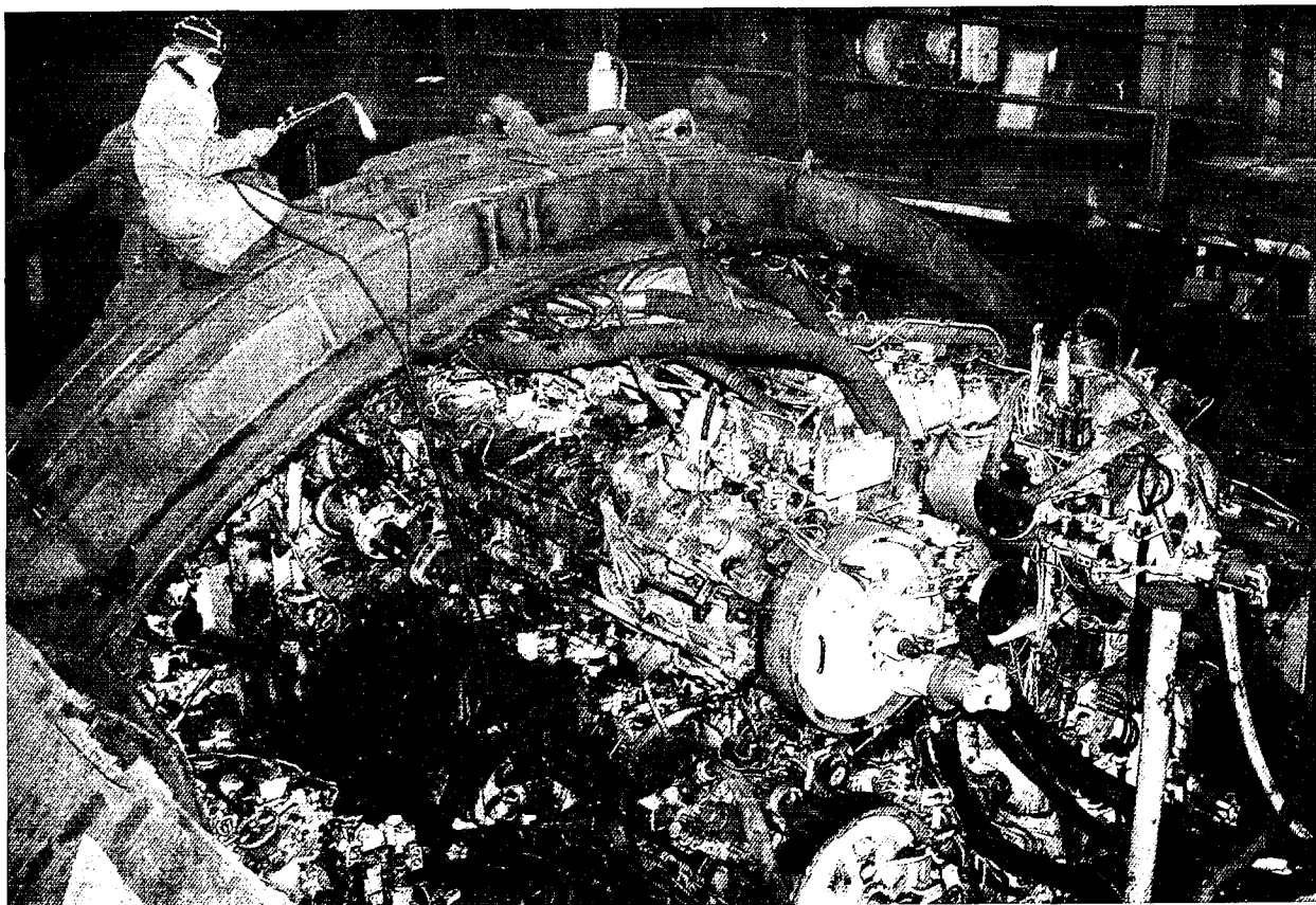
The decommissioning of Russian nuclear submarines is largely carried out manually in that the workers, as for example this man at the Nerpa shipyard, cuts into the hull using a blowtorch. The vessel pictured here is a Victor-I class submarine. The decommissioning of a larger Delta-I class submarine is estimated to take 32 000 working hours.
