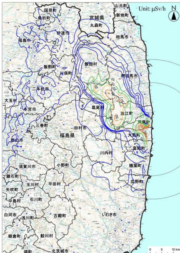
Figure 3A: Mapping of external dose rates ( \mu\text{Sv/h} ), published by MEXT on April 26, 2011
