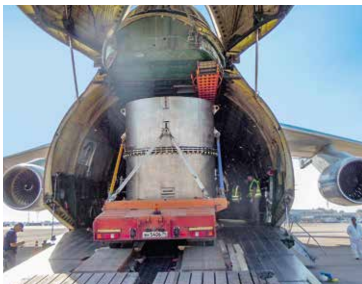
FIG. 2. A truck carrying a transport canister with irradiated liquid HEU fuel drives into a cargo plane for repatriation of the fuel to the Russian Federation.
