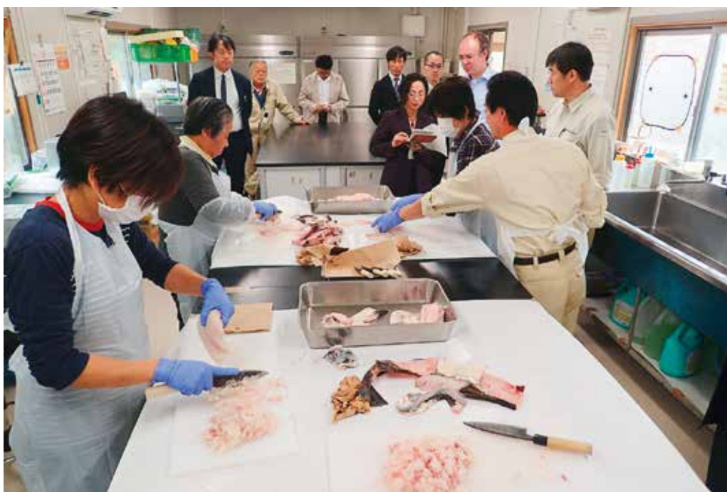
FIG. 2. Fish samples being prepared for an interlaboratory comparison of radionuclide measurements carried out by the Agency and laboratories in Japan.
