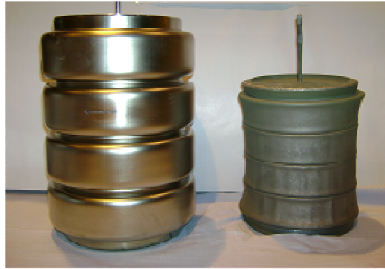
Figure 9. Hot isostatic pressing (HIP) for immobilization of impure plutonium in the UK. The container at the left is filled with powdered material. For plutonium disposal, it would be a mixture of plutonium, calcium, zirconium and titanium oxides. On the right, after 8 to 9 hours of hot isostatic pressing, the powder has been turned into 5 liters of solid ceramic. Source: UK National Nuclear Laboratory. 137
