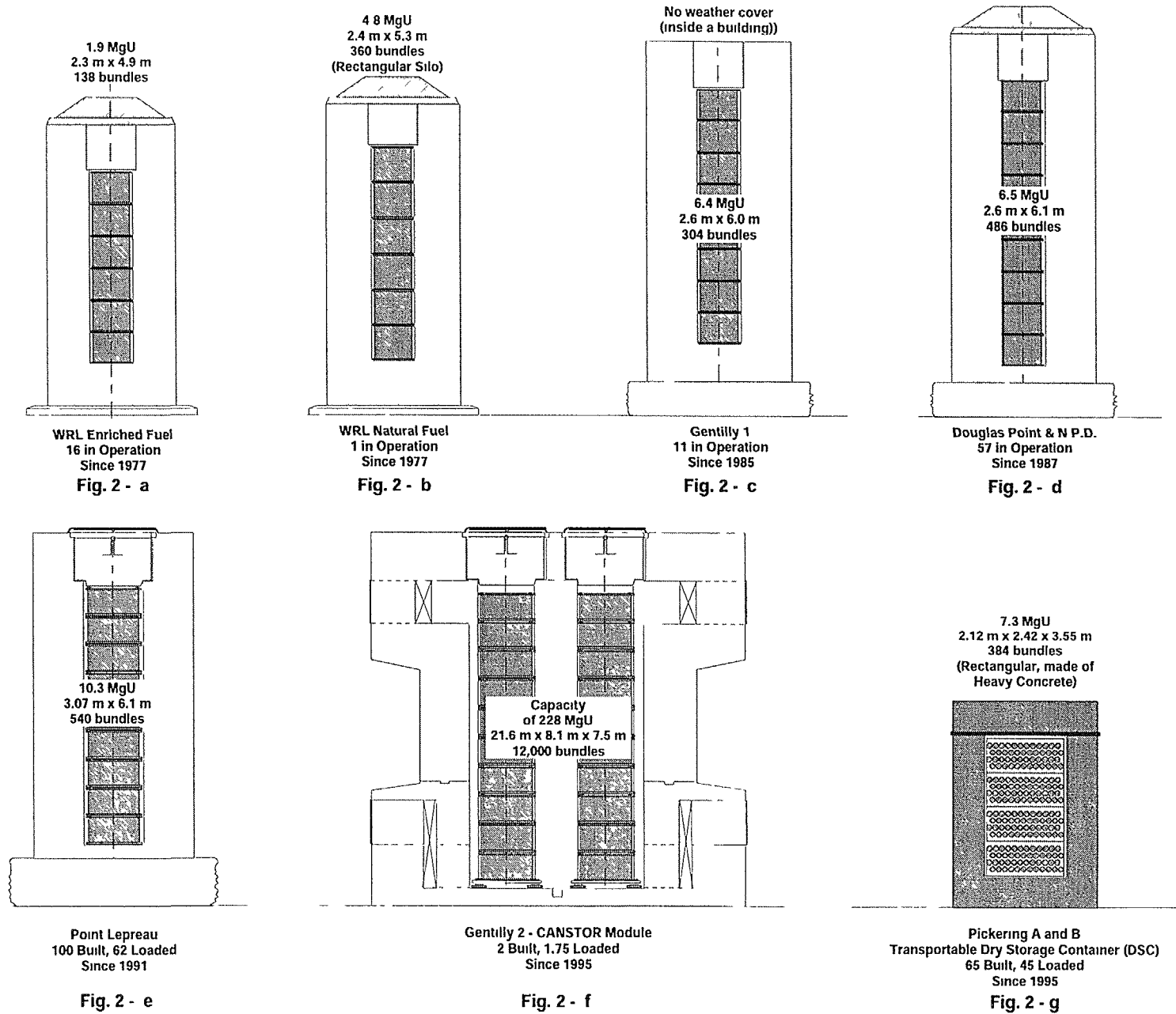
FIG. 2.0. Canadian concrete silos, module and cask (Data as of July 1997).
