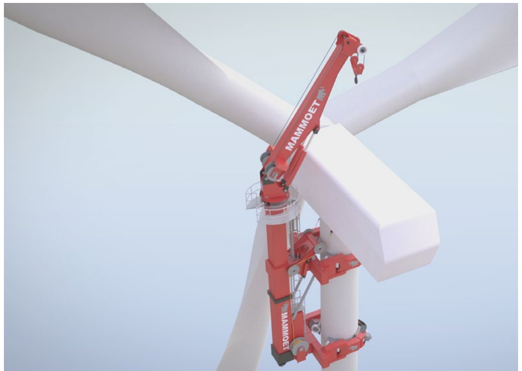
Figure 3. Impression of the self-anchoring maintenance crane. (Source: Mammoet Holding BV)
