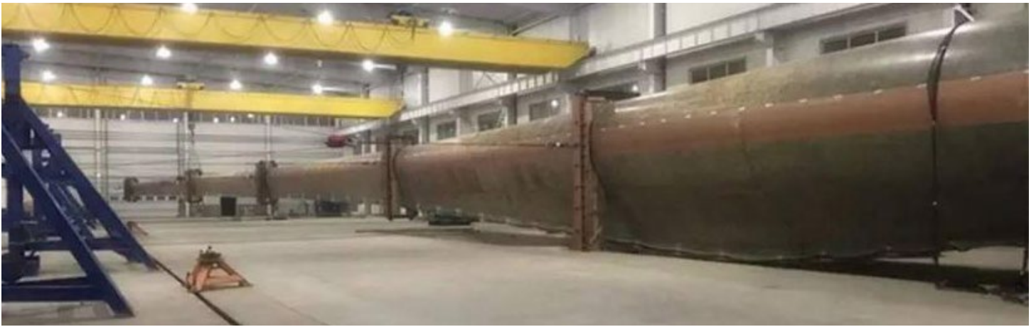
Figure 7. An 83.6-m long blade being tested in the China General Certification Center
