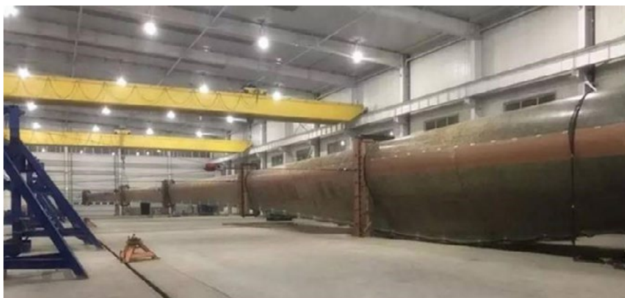
Figure 2. Natural frequencies and static tests of the longest blade (83.6 m)
