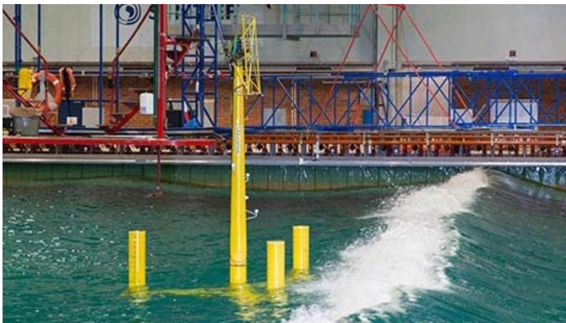
Figure 2. SINTEF's team has developed a unique test method called "Real-Time Hybrid Model (ReaTHM®)" as part of the LIFES50+ project (Source: Lifes50plus.eu) [16]
