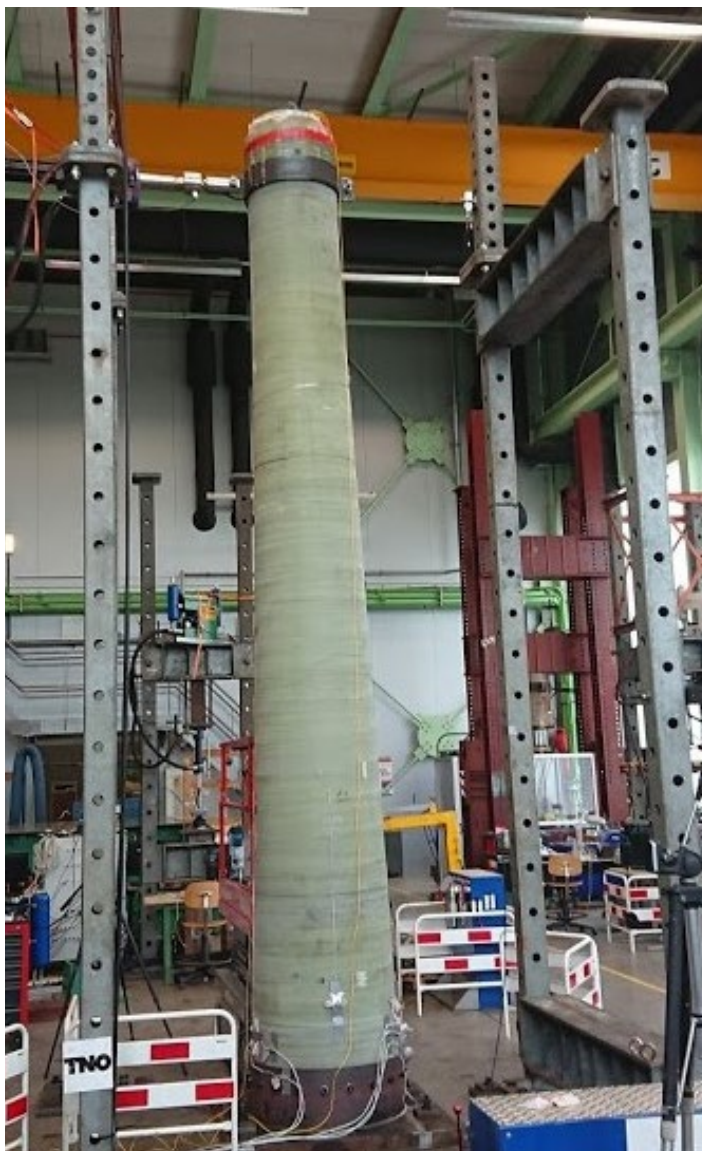
Figure 2. Scale model of the composite light weight tower (Source: Jules Dock Development BV)
