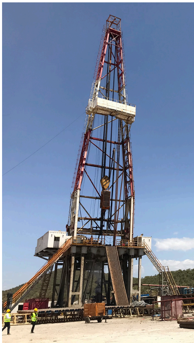
Drilling production wells in Olkaria, 2-3km below the surface © OLIVER JOHNSON
