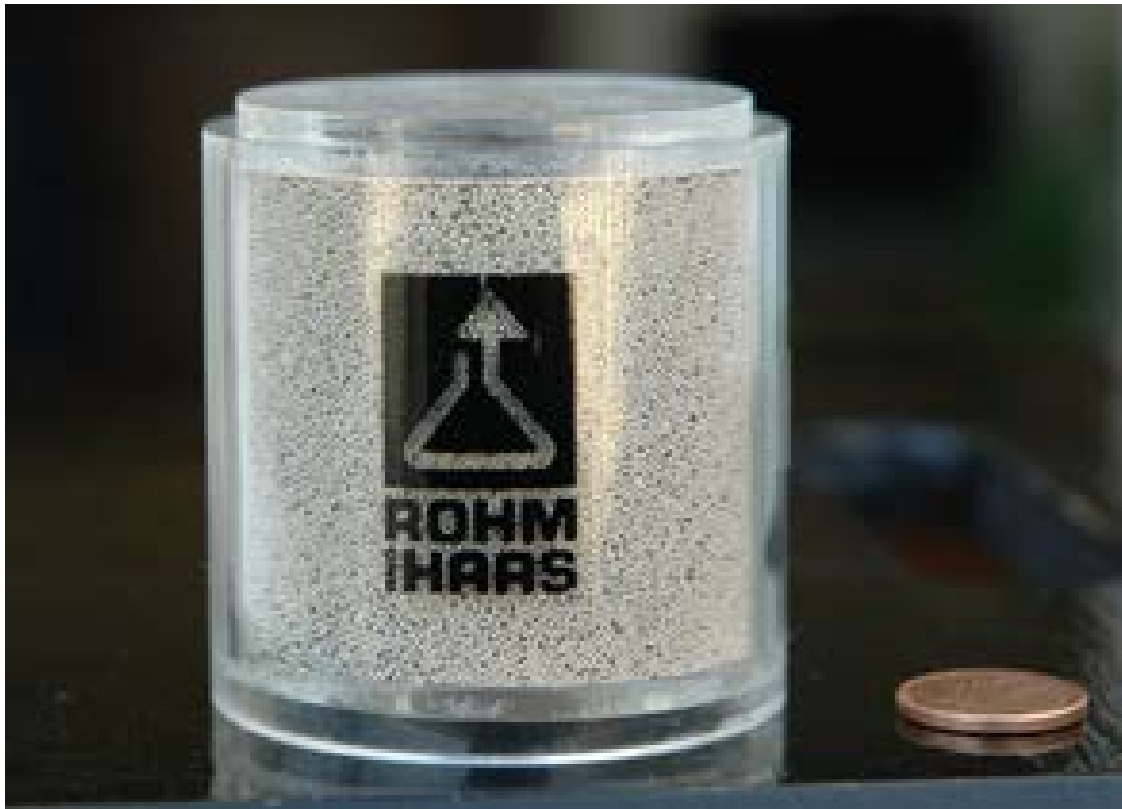
Figure 8: Sample of a macroporous cation resin
