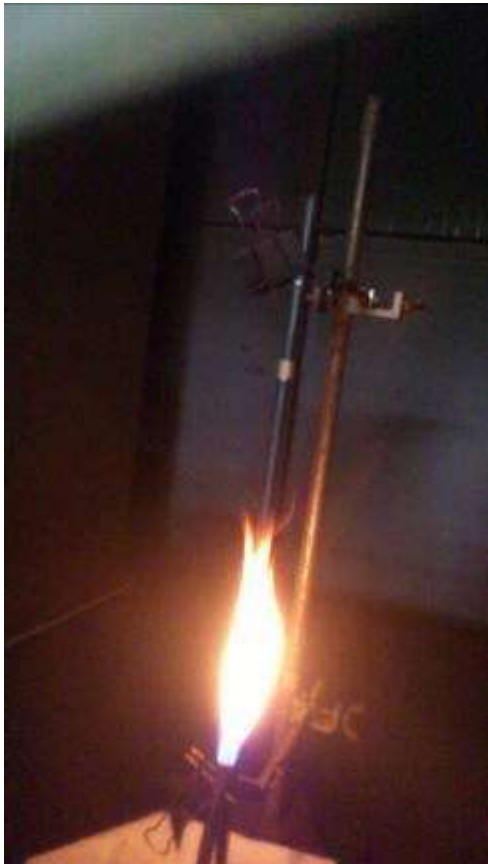
Example of verification test for self-extinguishing performance (UL vertical flame test)
