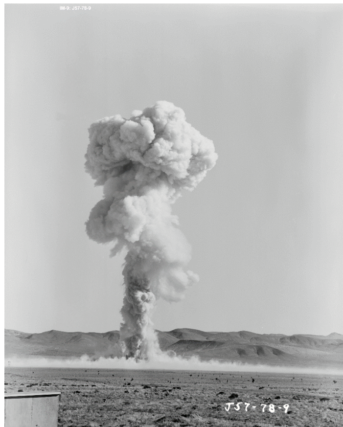
Figure 9: Shot Coulomb-C, one of Project 58s one-point safety tests
