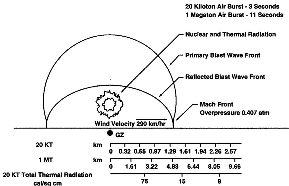
Figure 3-I. Chronological Development of an Air Burst
