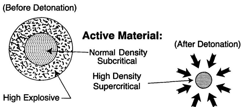
Figure 2-VIII. Implosion Assembly Principle
