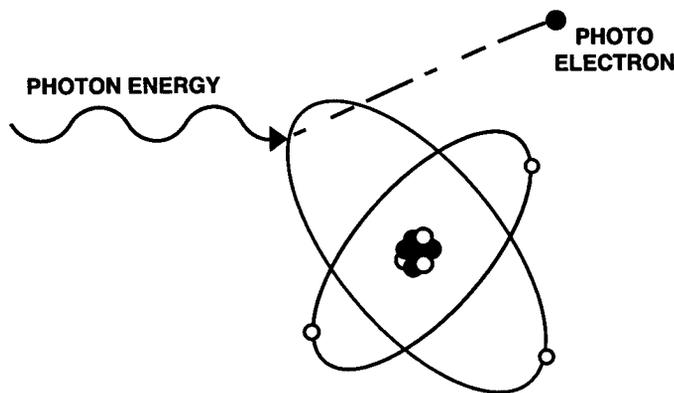
Figure 2-XIV. Gamma Interaction by Photoelectric Effect
