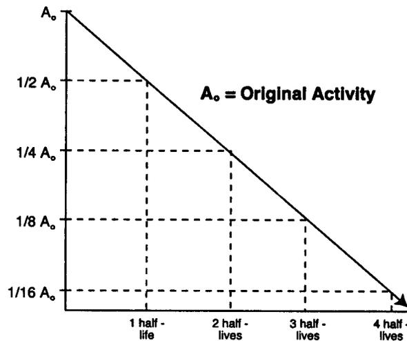
Figure 2-XI. Radioactive Decay Plotted in Semilogarithmic Form
