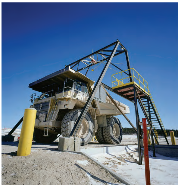
Figure 2.21. Overhead scanning of mined rock to classify ore and segregate potentially problematic waste rock for appropriate disposal, McClean Lake
