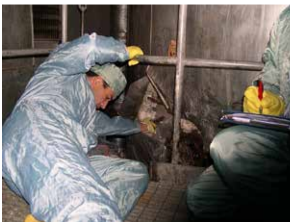
Figure 9.5: Steam generator radiological characterisation
