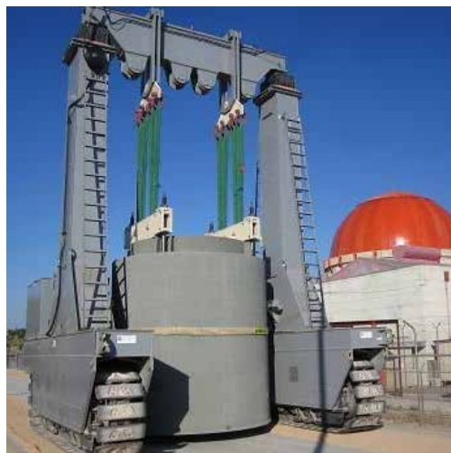
Figure 9.12: Transport of HI-SAFE cask to independent spent fuel storage installations
