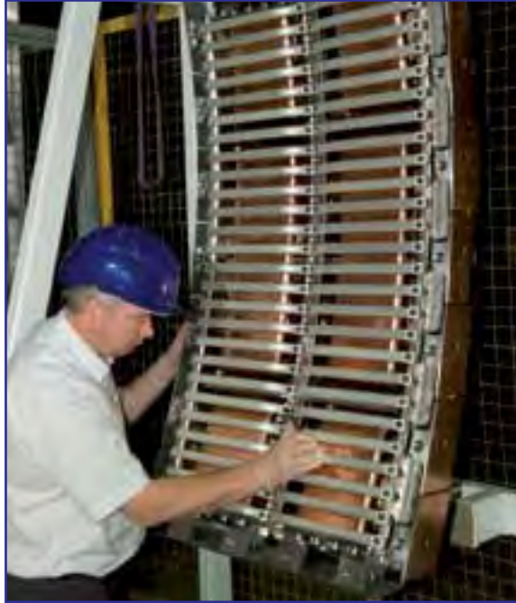
Figure 20: The JET's new ITER-like ICRH antenna during inspection
