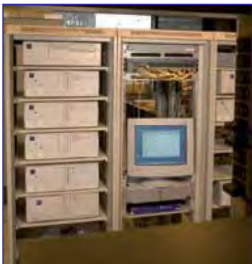
Figure 7: Part of the Real Time Measurement and Control System showing the analysis computers and an ATM network switch
