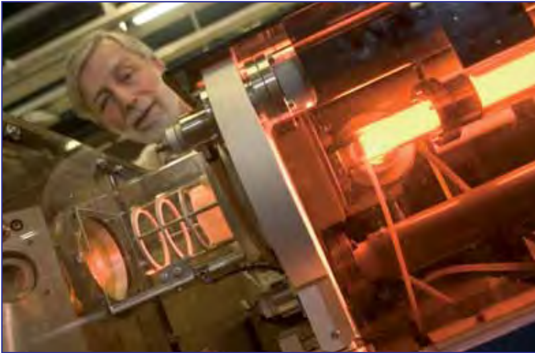
Figure 5: Laser Interferometer : measures refractive index for plasma density control.
