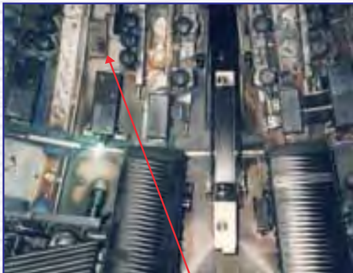
Figure 20: Electrode of the glow discharge system inside the JET vessel
