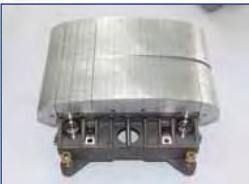
Figure 6: Two prototype beryllium tiles for the ITER-like wall project. Tile surfaces are segmented to relieve the stresses caused by thermal expansion and to reduce electromagnetic forces.
