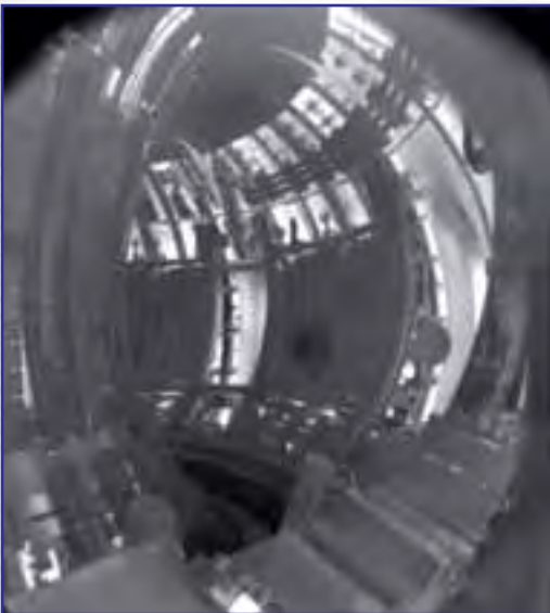
Figure 12: View into the JET vessel by the new wide-angle infrared camera
