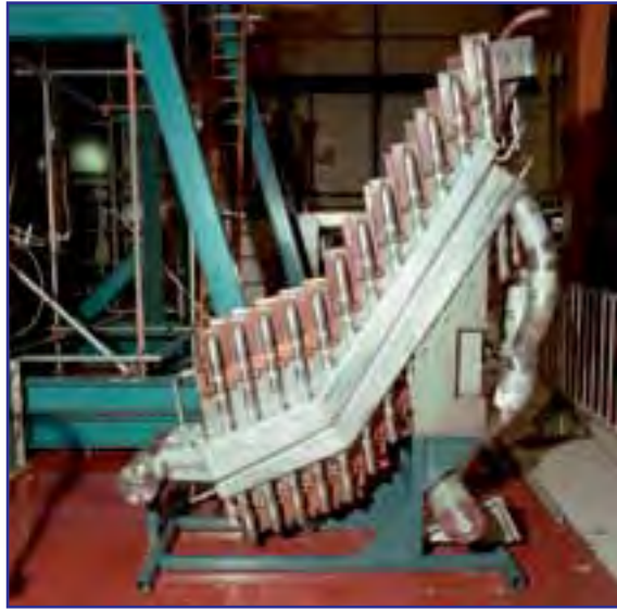
Figure 6: Ion dump of the JET Neutral Beam Injector
