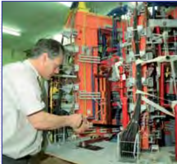
Figure 1: This scale model of JET was originally used for design tests of new components. Made redundant by 3D computer design environments, half is now exhibited in the JET foyer and the other half has been donated to the British Science Museum.
