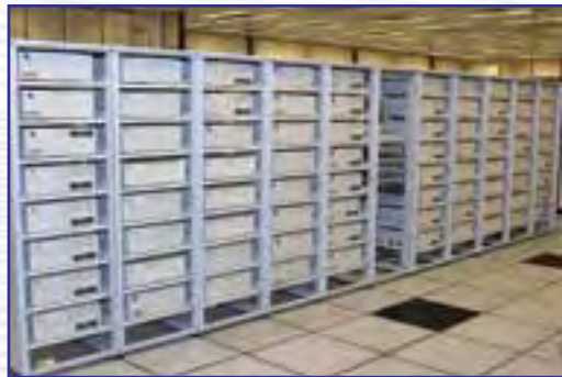
Figure 7: Today, the analysis of JET plasmas relies on clusters of high performance PCs. The photo shows part of the JET Analysis Cluster which consists of 165 Athlon processors running under Linux (as at February 2007)
