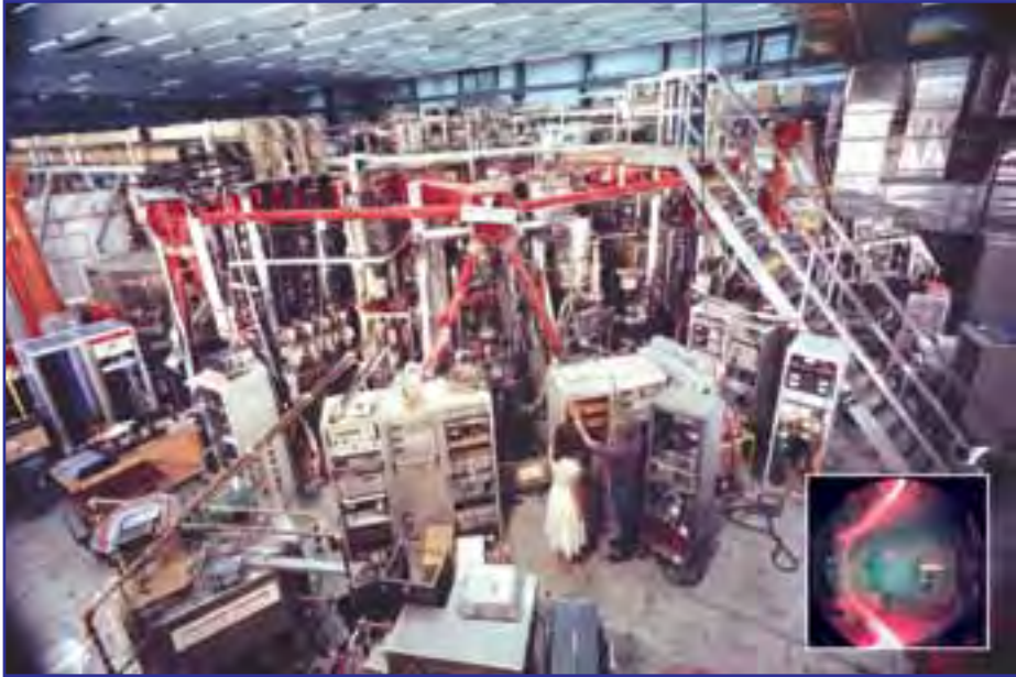
This picture shows the ASDEX tokamak where the H-mode was observed for the first time. The insert picture shows a plasma in ASDEX. At present, the Max Planck Institute for Plasma Physics in Garching operates a larger tokamak, ASDEX Upgrade, and is building a major superconductive stellarator Wendelstein 7-X in its new branch in Greifswald. The Max Planck Institute for Plasma Physics is an EFDA Associate and its experts are also significantly involved with JET work, both on-site and remotely. Photo courtesy of Max Planck Institute for Plasma Physics.
