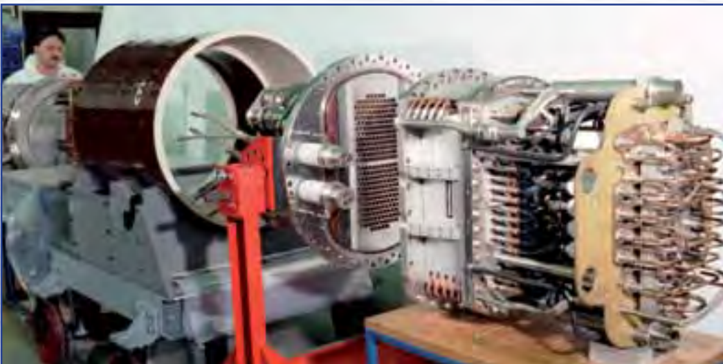
Figure 4: Assembly of one of the sixteen ion sources for the JET NBI system
