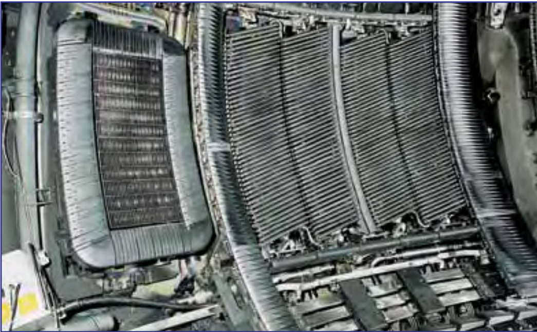
Figure 14: LHCD and ICRH antennas in JET vacuum vessel (LHCD grill in frame in left, next to it four slotted launchers of ICRH)
