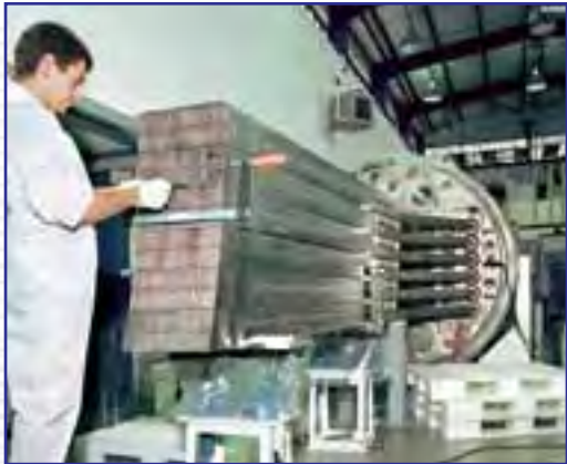
Figure 18: Completion of the LHCD antenna known as "multijunction grill"
