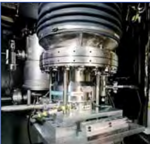
Figure 12: Turbomolecular pump at JET and its turbine rotor
