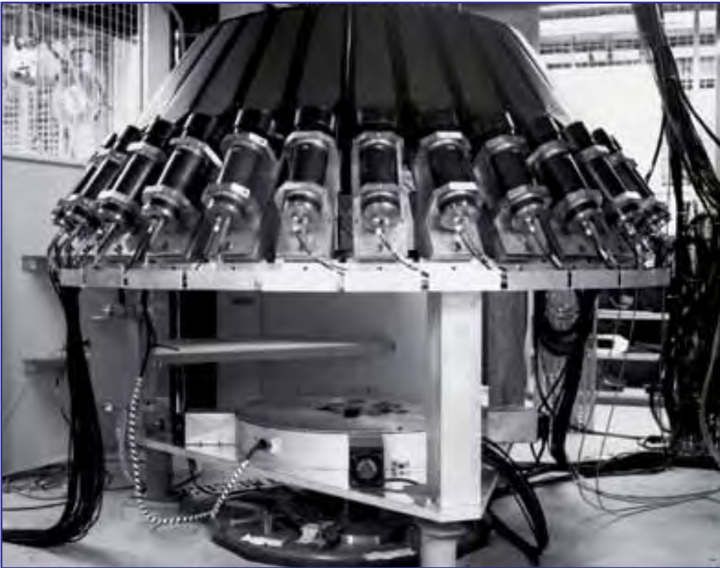
Figure 6: TOFOR assembly in the JET's roof laboratory (Photo by J Polverini and L Antalova)
