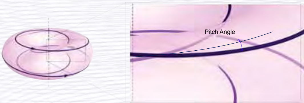
Figure 6: Near the plasma edge the magnetic field line pitch can be very low. The pitch angle is typically a few times smaller than in the image above
