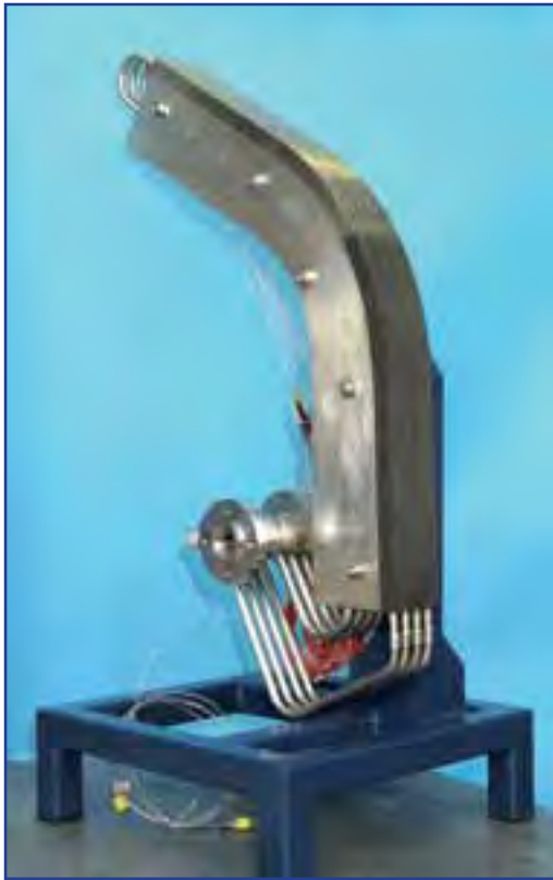
Figure 15: As a part of the ITER R&D projects, this ITER divertor target mock-up was manufactured by Plansee GmbH. High melting temperature and high energy threshold for sputtering are attractive features of tungsten (the top part of the mock-up consists of W brush armouring). Tungsten, however, due to its high atomic number presents a burdensome plasma impurity. Carbon Fibre Composite tiles (CFC, applied in the bottom part of the mock-up) are popular due to their unique thermal resistance, however, in fusion plasmas they suffer from hydrogen absorption and chemical sputtering. Image courtesy of ITER.
