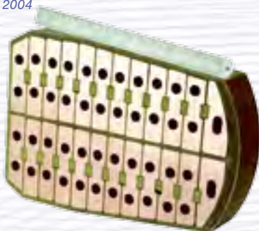
Figure 4: Photo of the JET toroidal coil in cross-section showing holes where the cooling liquid circulates
