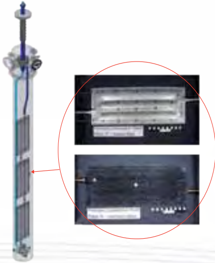
Figure 8: New pumping cryopanel: schematic drawing with cryosorption panel before coating with activated charcoal and after coating.
