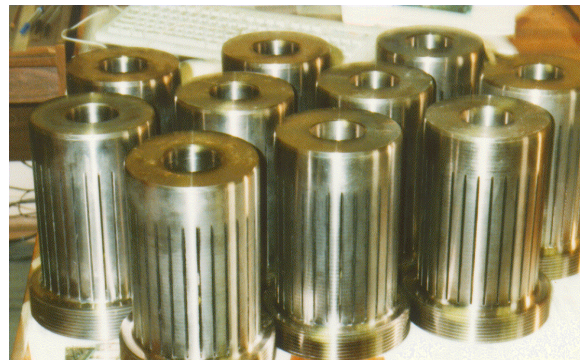
Figure 5.4-1 Flexible Mechanical Attachments made of Ti-Alloy (RF)
